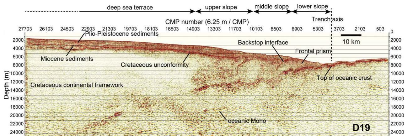
**Fig.1** Prestack depth migrated section in the central Japan Trench. In each panel, the vertical dotted line indicates the location of the trench axis (Kodaira et al. 2017).
