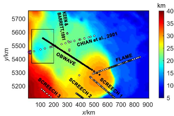
**Figure 2.** Moho depths from the density anomaly Moho-proxy from the 3-D gravity inversion in this study. The white points show the seismic survey lines which were incorporated directly into the inversion as constraints and the black points show the seismic survey line which were deliberately not used as constraints but were used to gauge the quality of the inversion results.
