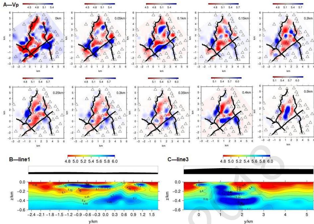
**Figure 2.** P-wave velocity structures at different depths and two vertical depth sections (line 1 and line 3).
