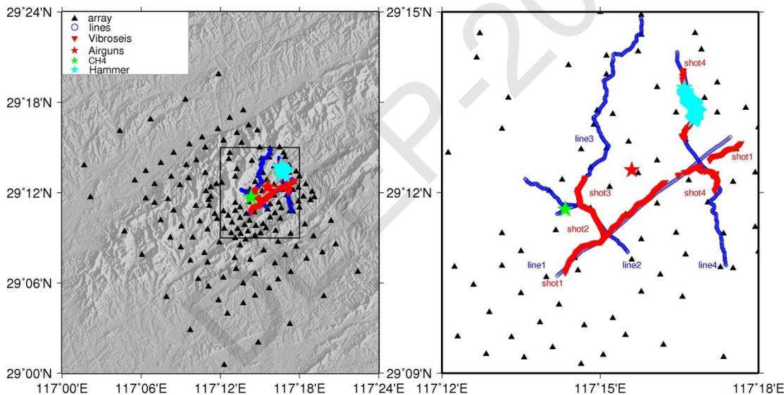
**Figure 1.** Excitation sites and station distribution for the Jiangxi Experiment. The red, green, blue stars represent the Airgun (215 shots), CH<sub>4</sub> (1 shot), and Hammer (44 shots) excitation sites, respectively; Red inverted triangles represent the Vibroseis excitation sites (738 shots); Black triangles and blue circles represent dense array and profiles, respectively;
